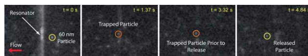
Fig. 8 Trapping of nanoparticles on photonic crystal resonator. The waveguide is excited at the resonant wavelength while 60-nm particles flow through a microfluidic channel running over the resonator and the waveguide. The yellow circle tracks the 60-nm particle which is trapped (indicated by orange circles) on the resonator. Turning the laser power off releases the particle from the trap. Reprinted with permission from Mandal et al. 56 Copyright 2010 American Chemical Society.
